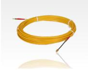
Polykat® fibreglass profile Ø 3,0 mm with integrated copper wires fitted with rod end with external M5 thread flexible guide head Ø 7 mm and pulling eye included
