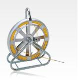
**2in1 concept: cable pulling device with detection function Polykat®** fibreglass profile Ø **4,5** mm with integrated copper wires fitted with rod end with external M5 thread and attached flexible guide head Ø 7 mm, connection box for connecting transmitter (1 connection) galvanized steel frame with aluminium reel Ø 400 mm
